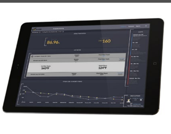
Figure 2. The dashboard displays hot water information, steam loss data and alerts.
